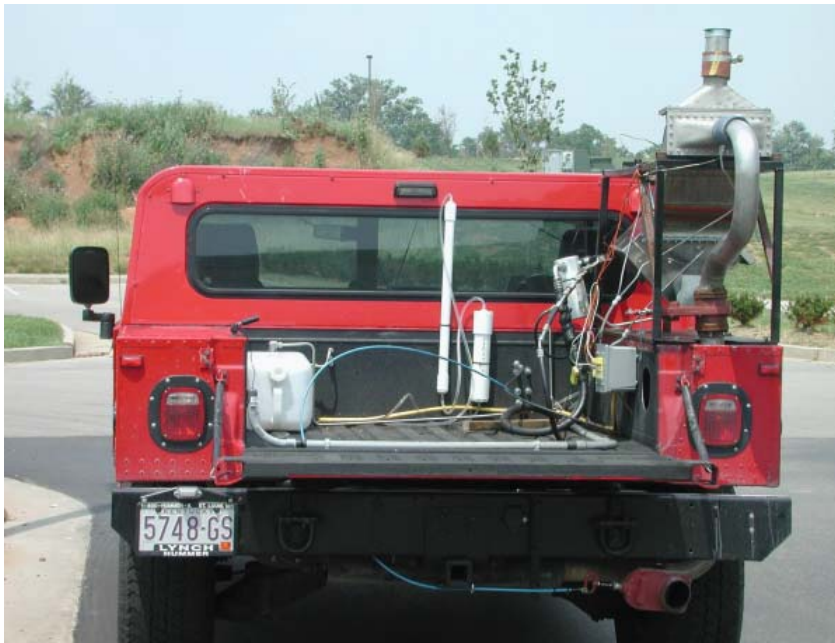
Figure 4 On-Board Water Recovery Unit
